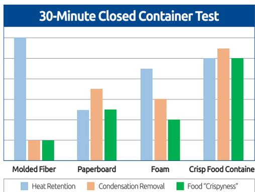
The graph on the left shows the results of tests performed at multiple locations of two leading national restaurant chains. While molded fiber performed the best in heat retention, it scored poorly in condensation removal and maintaining food texture. The best overall performance was delivered by the “Crisp Food Container.” The Crisp Food Container by Anchor Packaging of St Louis, MO is a patented technology currently in use at over 10,000 stores.
